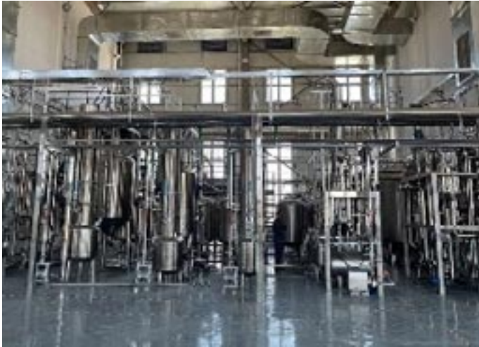
Picture 1: Industrial scale chromatographic system for sugar syrup purifications
